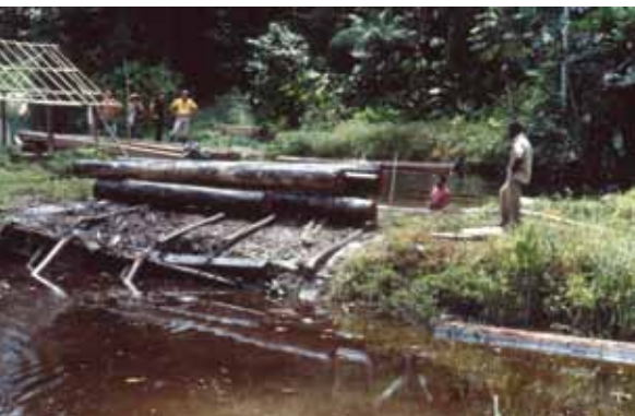
Photo 2.2. Virola spp. (Baboen) stems are pulled over a little dam, which separates two water basins with permanent different water levels. Coesewijne, Suriname, 1982. (Photo P. Schmidt)
